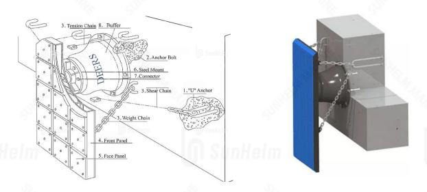
A SHD cone fender system includes rubber fender, steel frontal panel, face pad, fasteners, cast-in anchors, chain systems, etc.
