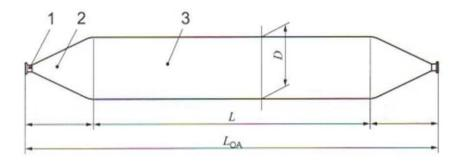
The core indicators of ship launching airbag quality comes from Rated Working Pressure, Bearing Capacity and Minimum Burst Pressure. These datas are calculated by specific calculation formulas. Another important indicator is SUNHELM ship launching airbag safety factor could reach at least 4.5 times. The formula is as follows:
